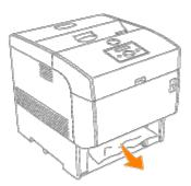
11. If jammed paper cannot be found, pull down the blue cover along the top of the hole where the tray cartridge was in the printer, and pull the jammed paper out carefully. Close blue cover after removing jammed paper.
