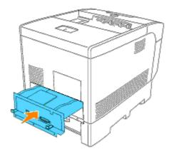
8. Tighten the three screws on the controller card from the back side of the printer.
