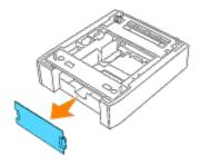
4. Gently pull out the tray of the optional 500-sheet tray module until it stops. Hold the tray with both hands, lift up the front slightly and remove it from the tray module.
