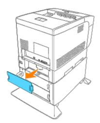
3. Pull the printer's tray out until it stops. Hold the tray with both hands, lift the front slightly and remove it from the printer.
