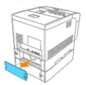
4. Pull the printer's tray out until it stops. Hold the tray with both hands, lift the front slightly and remove it from the printer
