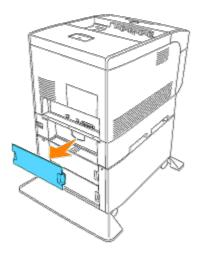
5. Pull the printer's tray out until it stops. Hold the tray with both hands, lift the front slightly and remove it from the printer.
