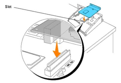
6. Align the two protrusions with the holes on the controller card, and then tighten the two screws from the back side of the controller card.
