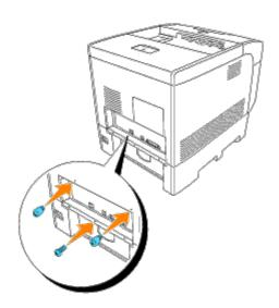
9. Reattach the paper tray cover to the back of the printer.
