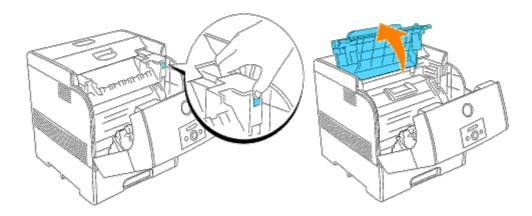
3. Grab the imaging drum by the handle, and pull it up and out.
