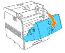
2. Push the button as shown in the following illustration and open the imaging drum cover.
