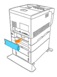
9. Pull the printer's tray out until it stops. Hold the tray with both hands, lift the front slightly and remove it from the printer.
