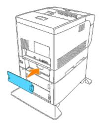
9. Peel off the peel-off paper on the double-sided adhesive tape on the cable hook, and affix the cable hook on the back of the printer.
