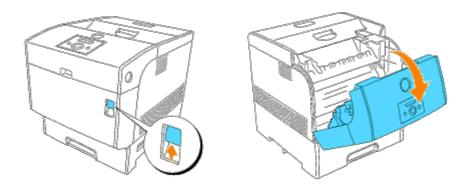
2. Push the button as shown in the following illustration and open the imaging drum cover.
