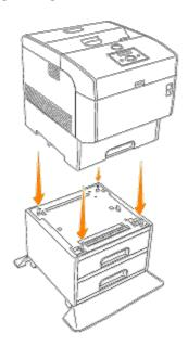
**NOTE**: Be careful not to pinch your fingers when lowering the printer onto the optional 1000-sheet tray module.
