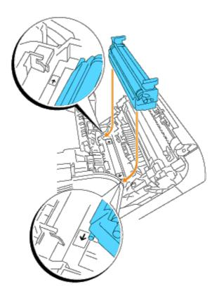
3. To lock the transfer roller into the printer push down the tabs until you hear a click.
