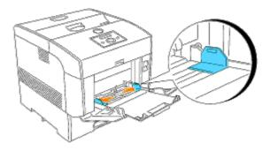
3. Insert all media face down and top edge first into the multipurpose feeder.
