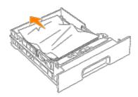
3. Pull the jammed paper out carefully to avoid tearing it.
