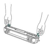
6. Align the arrow marks on the transfer roller to the marks on the printer, and gently push the roller into the printer.
