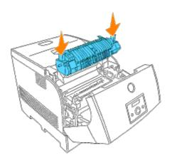
2. Completely push down the fuser by holding the knobs at both ends of the fuser until the levers next to both ends of the fuser return to their original position.
