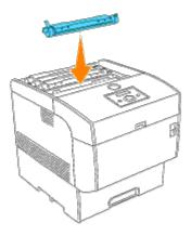
7. Grip the levers at each end of the toner cartridge with your fingers, then push down firmly to rotate the levers forward.
