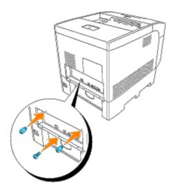
8. Reattach the paper tray cover to the back of the printer.
