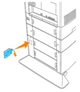
14. Plug the power cable into the power cable connecter at the back of the printer, wind the power cable onto the cable
