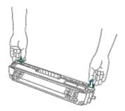
2. Align the arrow marks on the transfer roller to the marks on the printer, and gently push the roller into the printer.
