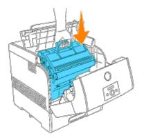
3. Pull the protective cover on the imaging drum straight up to remove it.
