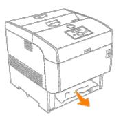
4. If jammed paper cannot be found, pull down the blue cover along the top of the hole where the tray cartridge was in the printer, and pull the jammed paper out carefully. Close blue cover after removing jammed paper.
