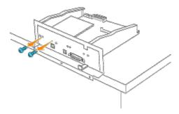
6. Hold the multi protocol card and remove it from the controller card.
