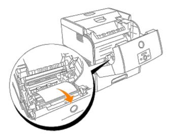
**NOTE:** If a paper jam occurs in the fuser area, a sheet of paper may already have been fed from the tray. Make sure there is no paper remaining inside the printer, using step 8 through 14.
