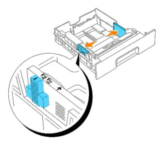
3. Squeeze the length guide and slide it to the edge of the tray.
