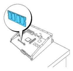
6. Push the memory card into the slot firmly.
