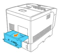
5. Place the controller card on the table so that its edge hangs over the edge of the table and the controller card is horizontal. Push the clips on both sides of the slot outward. Remove the memory card from the slot.
