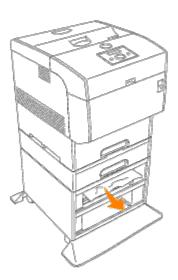
4. Push the front latch up and fully open the front cover. Confirm that there are no scraps of paper remaining inside the printer.
