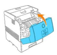
5. If a paper jam message is displayed, push the front latch up and fully open the front cover.
