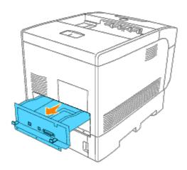
$5. \ \ Replace$  the two screws from the back side of the controller card.
