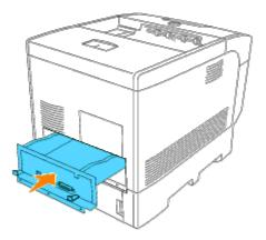
8. Tighten the three screws on the controller card from the back side of the printer. The two screws on the upper side are different in shape from the one on the lower side. Be careful not to confuse them.
