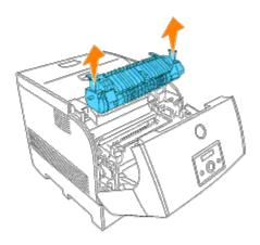
5. Unpack a new fuser, grip the fuser by the knobs, align it with the slots in the printer, and slowly push it in.
