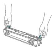
4. Align the arrow marks on the transfer roller to the marks on the printer, and gently push the roller into the printer.
