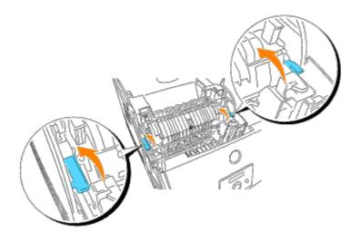
4. Grip the knobs and gently lift the fuser out of the printer.
