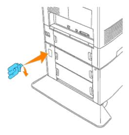
10. Plug the power cable into the power cable connecter at the back of the printer, wind the power cable onto the cable hook as shown in the graphic, and lightly pull the power cable. Then, plug the other end of the cable into the grounded outlet.
