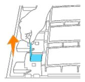
NOTE: Pull the toner seal straight up. Pulling the toner seal diagonally may tear the seal.
