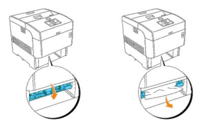
5. Push the front latch up and fully open the front cover. Confirm that there are no scraps of paper remaining inside the printer.
