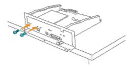
7. Insert the controller card into the printer.
